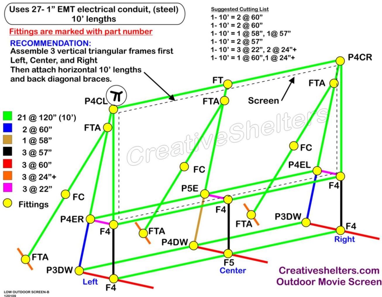
Figure 1 Assembly and cut list drawing for KODSCREEN2
