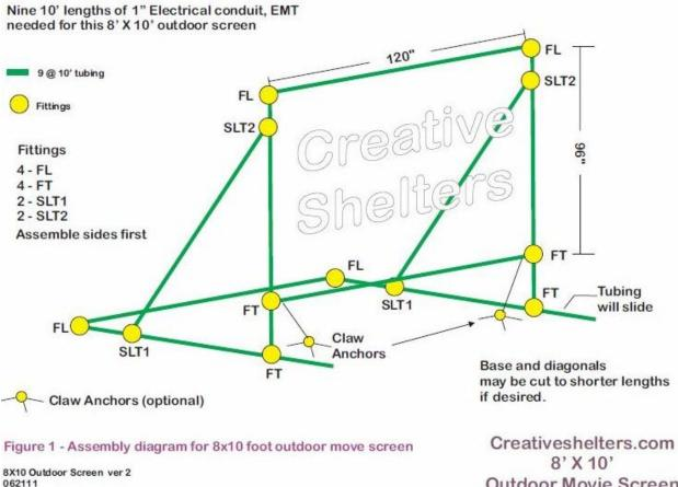
Figure 1 - Assembly diagram and tubing cut list for 8x10 foot outdoor movie screen
